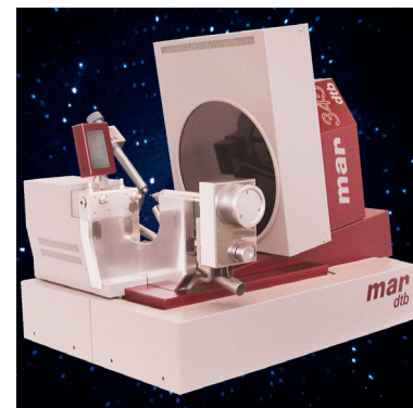
Figure 3: mar345 image plate detector mounted on a “desktop beamline”
